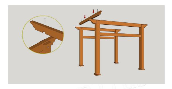
8. After all the beams are fixed, fix the posts and base support with 5.5 \* 75 drilling screws at 200mm and 600mm from the ground outside the posts.
