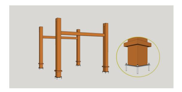
4. Insert the 200 \* 80 mm Crossbeam into the slotted post and adjust the length before and after.
