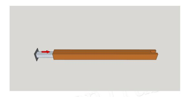
2. Fix the base support and concrete with expansion screws, and insert into the post skirt.
