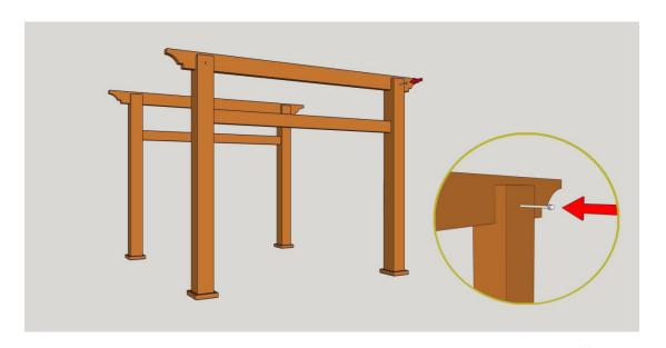
6. Use  $\Phi$  5mm twist drill to drills drainage holes at the slot of 160  $\star$  80mm beam.
